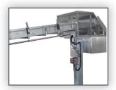
Start-up head with height adjustment, strand breakage monitoring and safety guard
