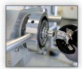
Single-hand locking Simple cutter hub replacement
