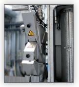
Agglomerate catcher with a pneumatically operated gate valve (seal without sealing material) and automatic ejection (optional)
