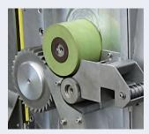
Cantilevered design of cutting and draw-in section
