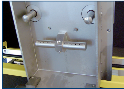
Cutting area cooling
