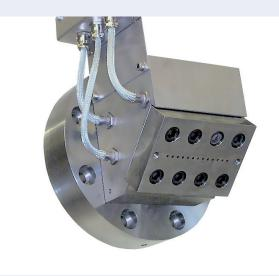
Electrical heating with cartridge heater
